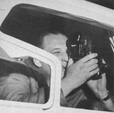
Sighting through a plane's Plexiglas window sometimes results in slight errors. The errors can be checked out and corrections made during a local night flight. The photograph shows Schiff making a through-the-window sighting
