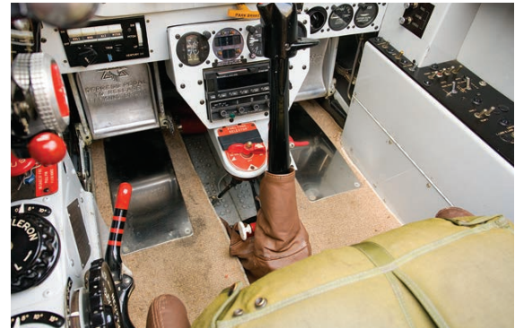
The three trim wheels (left) are clustered together, and the rudder pedals (below) are adjustable fore and aft for tall and short pilots.
